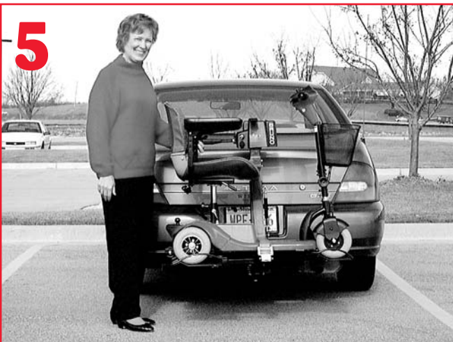
5 Place scooter on platform, press switch to raise and secure with belt.
