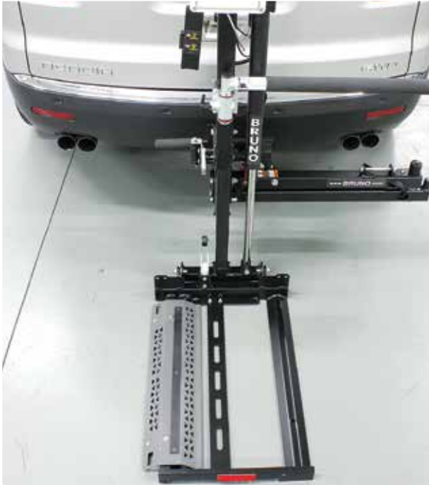
HTP Mid Wheel Drive (MWD) option shown accommodates MWD powerchairs with 10 in and 14 in wheels.
