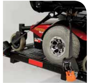
Retractable belt securement for powerchairs/scooters (ASL-250B).
