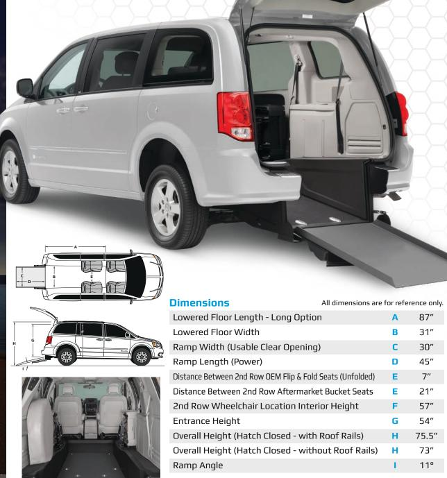
Due to manufacturing tolerances both with the OEM vehicle and the conversion components, all dimensions may vary slightly from those shown.
